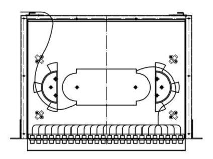
Fiber cable enters into the ODF by split & fix plate at back, and splices with pigtail inside the splice tray after passing through the fiber spool.
